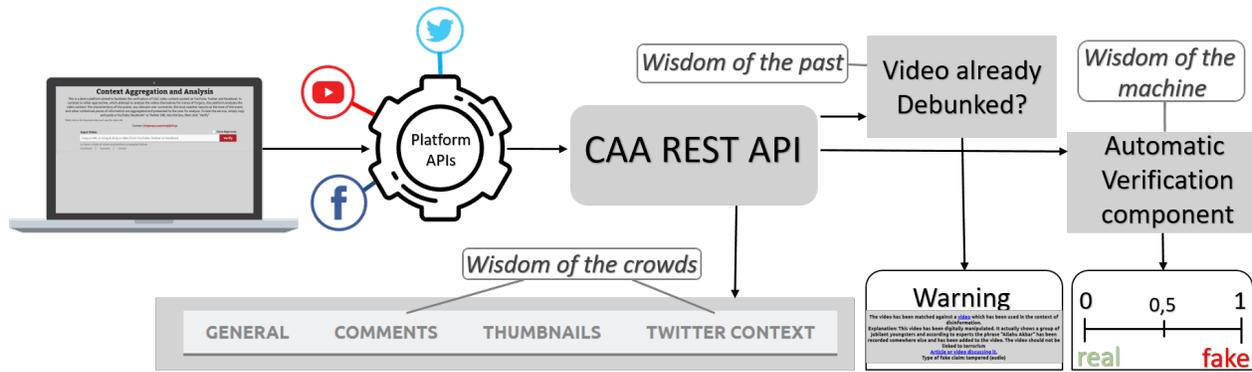
Figure 1: Context Aggregation and Analysis service pipeline.
